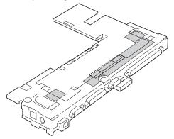
To remove the processor card, gently lift the area shown by A straight up. Do not pull the other areas.
